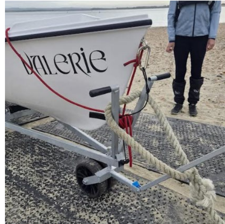
22. Attach winch rope over jockey wheel handle and onto trolley's handles. Ensure line and carabiner have secured Valerie, but you have flexibility for jockey
